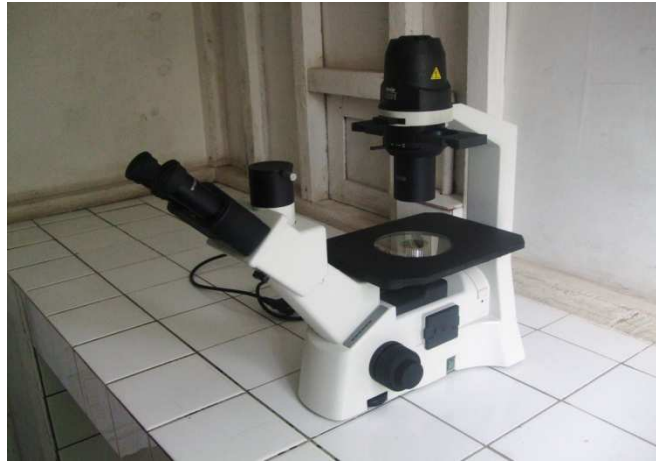
Figure 2 : Microscope inversé (Motic AE31)
